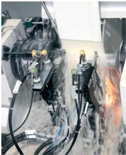
The diamond roll dresser is mounted on the grinding table. Dressing is effected via the X- and the Z-axes of the machine. The contour dressing system allows the generation of any required workpiece contour. Form and position tolerances of every diameter can be separately corrected by simply entering the values in the input mask of the control unit.
